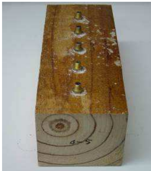
Figure 3. Timber blocks (10×10×30 cm) are in the position for testing and sample ports are 5, 10, 15, 20 and 25 cm from one end of the block and the other end is sealed with silicone.
