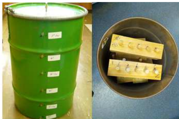
Figure 8. The fumigation chamber (47.8x40 cm id = 61 L) equipped with gas injection and sampling systems for laboratory scale trials.
