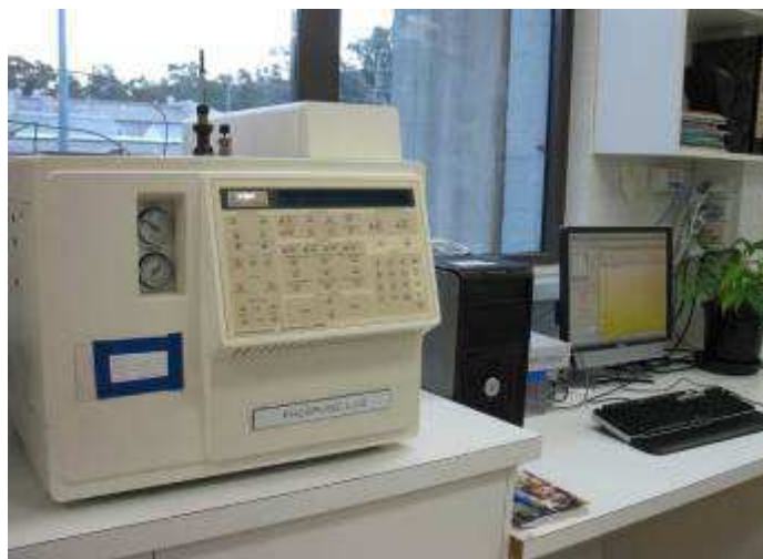
Figure 1. The concentration of EDN and MB in fumigation containers was analysed with Gas Chromatograph (GC) equipped with Flame Ionisation Detector (FIP)
